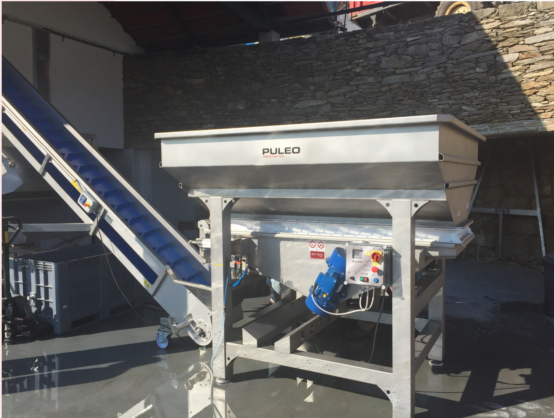
GRAPEO AND BELT ELEVATOR - SYMINGTON FAMILY ESTATES - PORTUGAL
